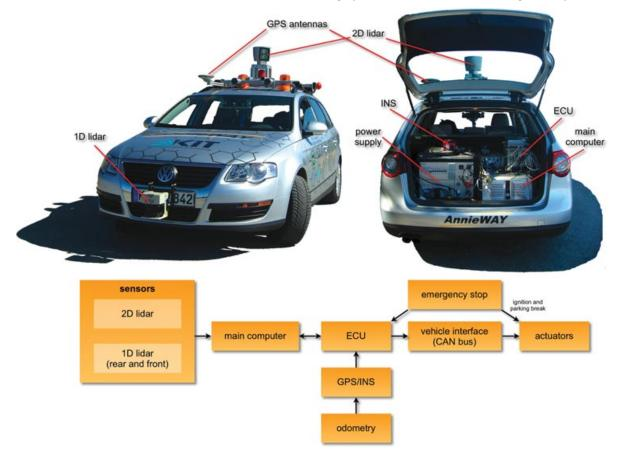
Figure 2. Architecture and hardware components of the vehicle.
