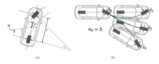
**Figure 17.** (a) Kinematic one-track model underlying both search graph and closed-loop control. (b) Search graph. Successors are generated for  $n_{\delta}$  discrete steering angles.
