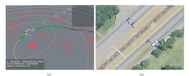
**Figure 24.** (a) Path planning in heavily occupied zone with mapper input (red) and sampled way points as output to the controller (green). (b) Recovery maneuver during final event; driven path is marked olive.
