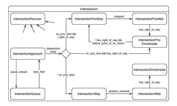
Figure 15. UML diagram of substate Intersection.
