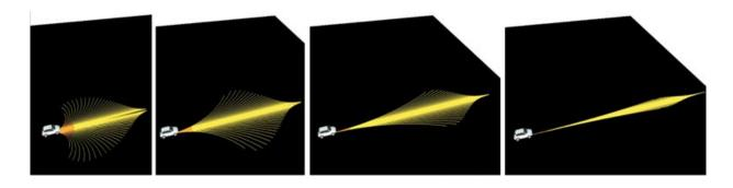
**Figure 9.** The reactive system uses a precomputed set of motion primitives that vary with the speed of the vehicle. As detailed in von Hundelshausen et al. (2008), those primitives are used to evaluate a vehicle-centered occupancy grid to avoid obstacles.
