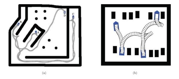
**Figure 19.** Some results of path planning on simulated map data. (a) Navigating large distances in a maze-like environment. Planning was from A to B, B to C, and C to D subsequently. (b) Some difficult parking maneuvers performed subsequently. Robot started on the right.
