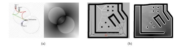
**Figure 18.** Cost functions. (a) RTR metric for three different starting positions. Left-hand side shows the minimum RTR paths; right-hand image the value of the RTR metric, densely evaluated on  $\mathbb{R}^2$  (bright: high value; dark: low value). (b) Voronoi-based cost function. (Left) Voronoi graph labeled with distance by Dijkstras algorithm. (Right) Voronoi-based cost function evaluated densely on  $\mathbb{R}^2$  by matching to the Voronoi graph.
