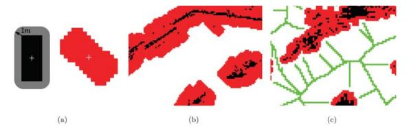
**Figure 16.** Configuration space obstacles. (a) A 1-m safety distance is added to the shape of the vehicle. Subsequent rotation and rasterization yields a convolution kernel for configuration space obstacle generation. (b) Result of convolving obstacle map with kernel from panel a. If the robot has the same orientation as the kernel and is placed in the red area, it must intersect with an obstacle. (c) Voronoi lines are generated as a set of eight connected pixels.
