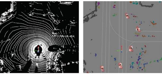
(a) High-resolution LIDAR data
