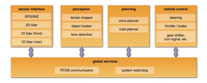
Figure 3. Overview of the software architecture and the information flow.
