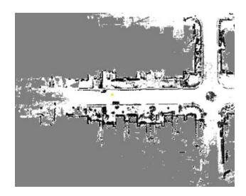
**Figure 4.** Example for the evidence mapping of 3D LIDAR data onto a 2D grid. Darker spots correspond to high evidence for an obstacle, and white cells correspond to drivable area. Unknown cells are gray.
